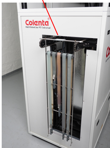
hanger loading section
